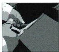
(2) Cut off the spacer rubber from both edges of the A-film.
