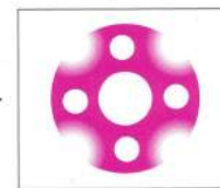
(5) Remove film and observe pressure distribution.
