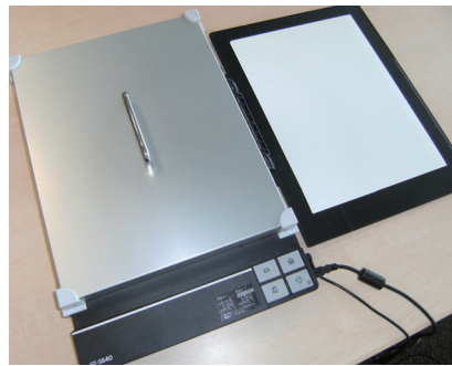
②Set UVSCALE on the scanner (recommended model) and scan the color sample.
